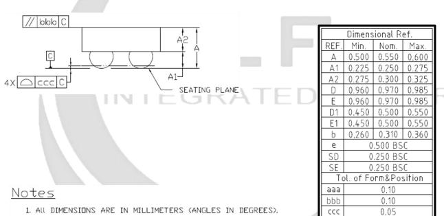
2. DIMENSIONING AND TOLERANCING PER ANSI Y14.5M-1994.
